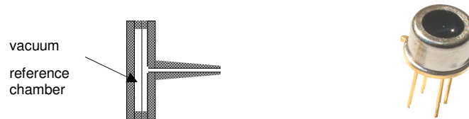
Fig 3, Principle of the absolute pressure sensor.
